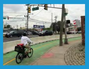
Protected Bike Lane Barrier Upgrades – To further enhance bicyclist safety and comfort, concrete jersey barriers and crash cushions are being installed wherever feasible along the existing protected bike lane network. This will protect cyclists from vehicular traffic with a durable, physical barrier and prevent vehicles from blocking the bike lane. Tuff Curb is also being evaluated for segments unsuitable for jersey barriers.
